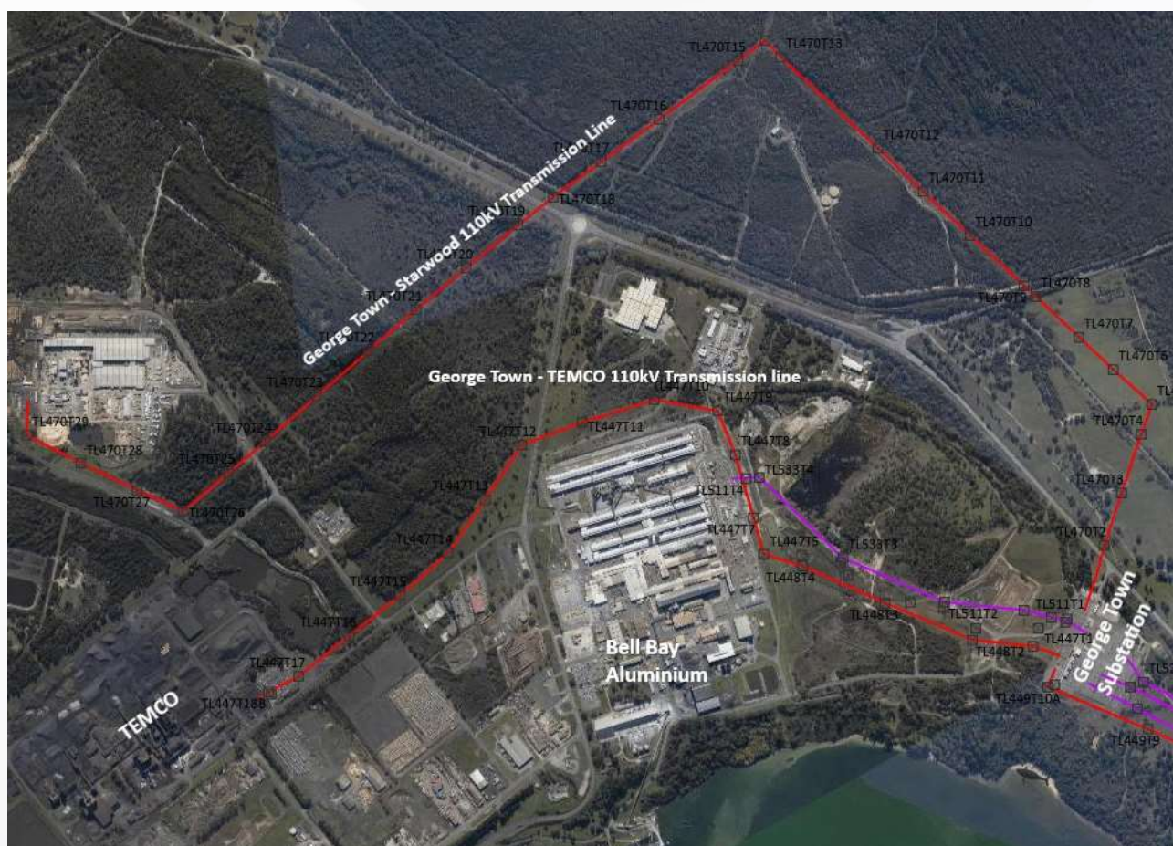
Figure 2: Bell Bay 110kV transmission network
